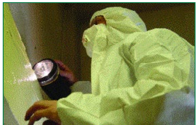
Figure 6.3 A torch being used to illuminate fine settled dust
