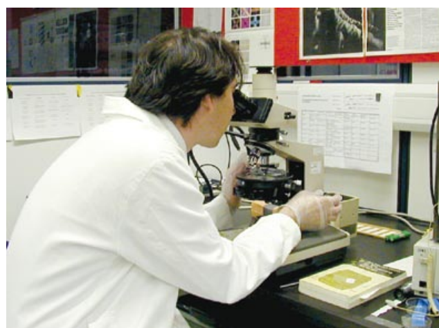
Figure 4.2 An analyst carrying out asbestos analysis
