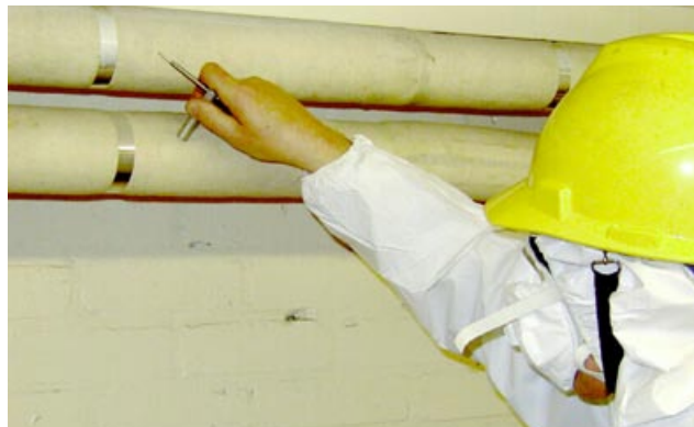
Figure 4.1 Analyst taking a core sample
