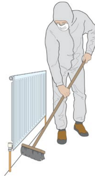
Figure 6.7 Analyst carrying out disturbance by brushing during clearing
